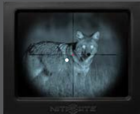
The rangefinder target is clearly visible on your viewing screen as a white dot, so you know the data it provides matches your intended target
